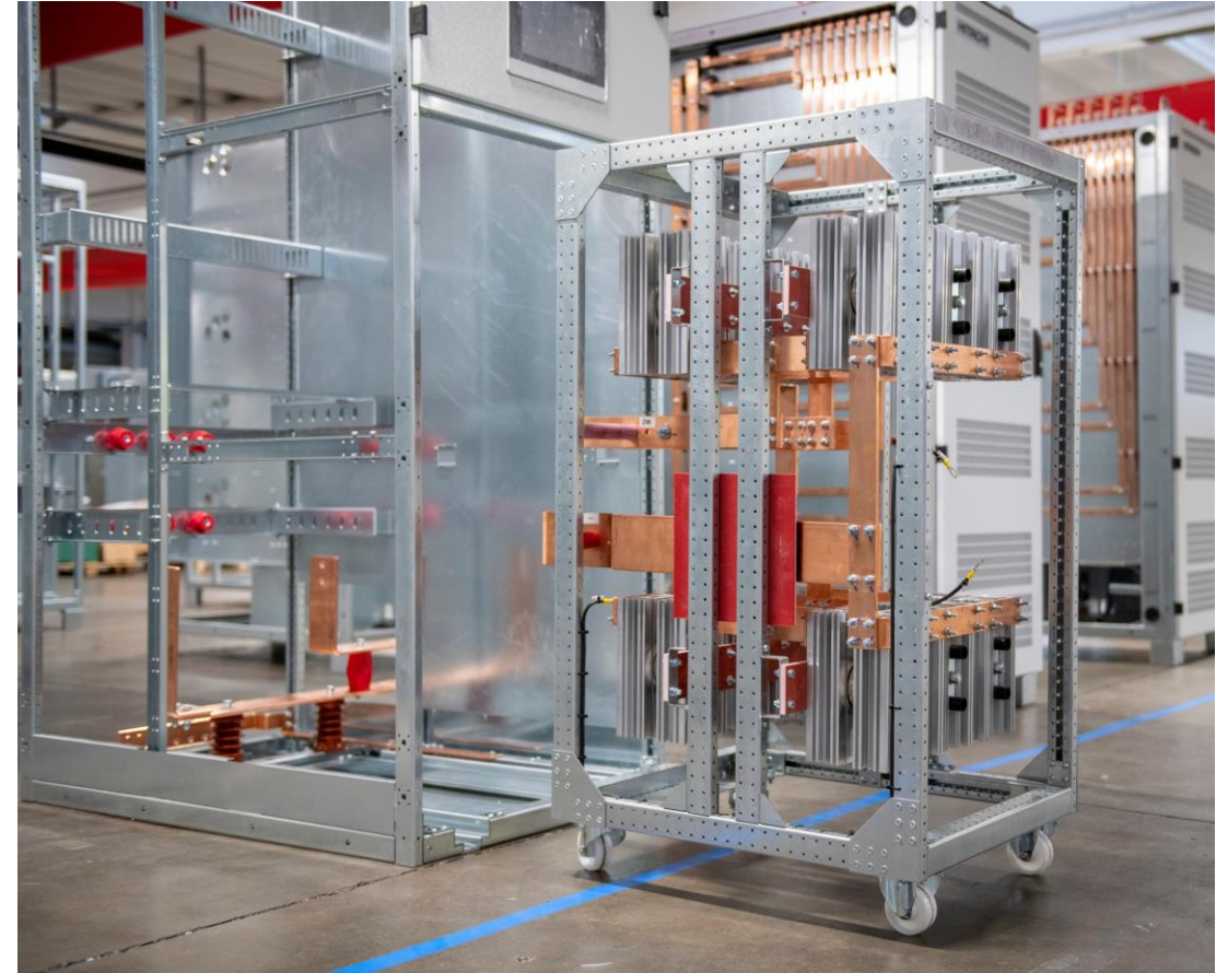
Movable rig for easy replacement of diodes
